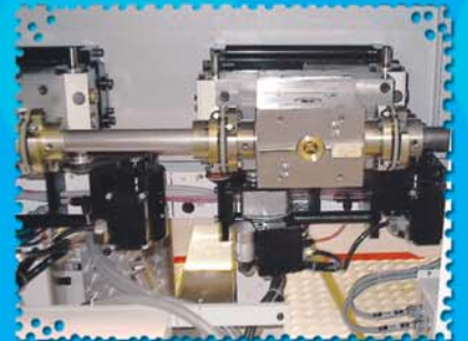
Advanced Tandler gear boxes on the DBX provide 360-degree motorized circumferential registration capabilities.
