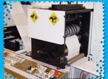
There are two individual die cutting stations and one sheeting or cross perforation station on the DBX with space for additional die cutting and/or punching units. The DBX die cutting stations feature removable anvil rolls of fully hardened steel and an advanced waste matrix removal system with stripping rollers and a rewind air shaft.
